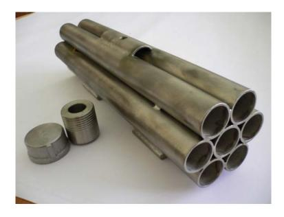
The tubes in each TRG vane bundle are welded at both ends at each point of tangency. Tube inlets and outlets are reamed to permit minimum pressure drop. Special spacer lugs on each vane bundle assure a perfect fit in the meter tube.
